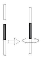
Fit the water-proof plate onto the lower supporting tube and then attach the lower supporting tube onto the motor body by screwing it in a clockwise direction.
